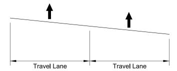
Figure 5-05: One-Way Tangent Crown
